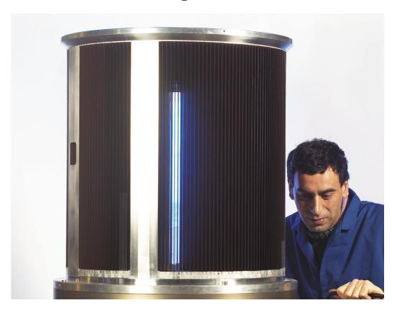
Euro Collimators have extensive experience in manufacturing oscillating radial collimators.
